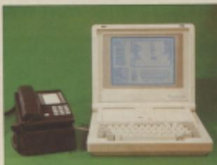
the React 320 Plus telephone, the system enables users to carry out all the functions of phoning directly from their computer, whether it is a BBC, Mac or PC.
